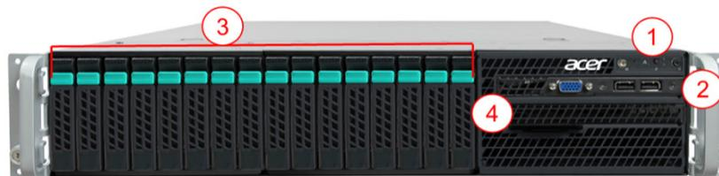
1. Power button, LED indicators: power, HDD activity, LAN, system ID
